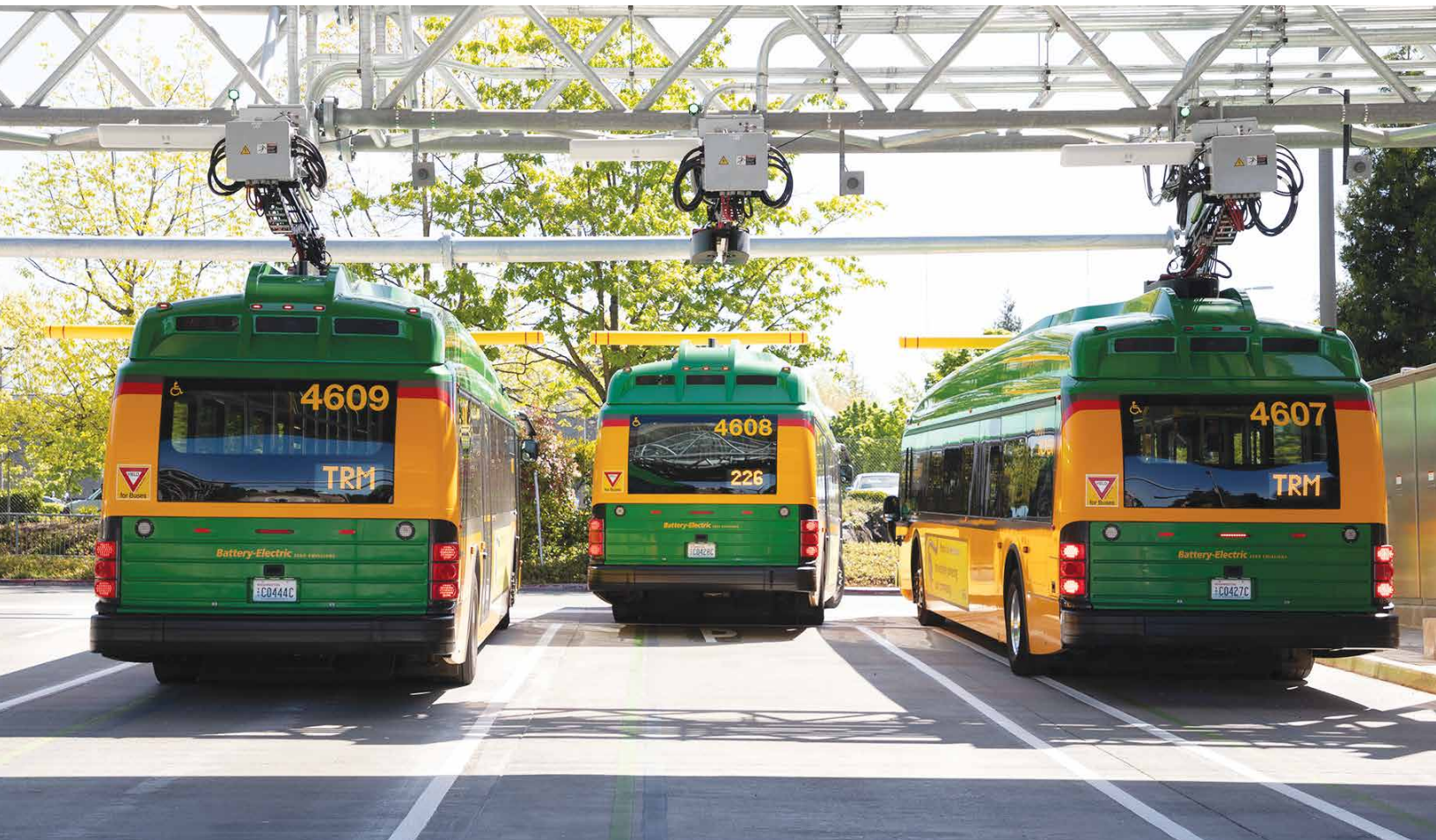
Battery electric buses charging at Eastgate Park-and-Ride.
