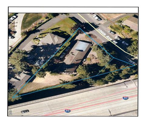
Bennett property boundary in blue. WTD needs a five foot permanent easement along the entire south property line parallel to I-90, and an an additional eight foot temporary construction easement along approximately a third of the south property line.
