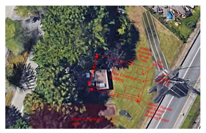
Figure 5. Risdon Well Site Wellhead Treatment
