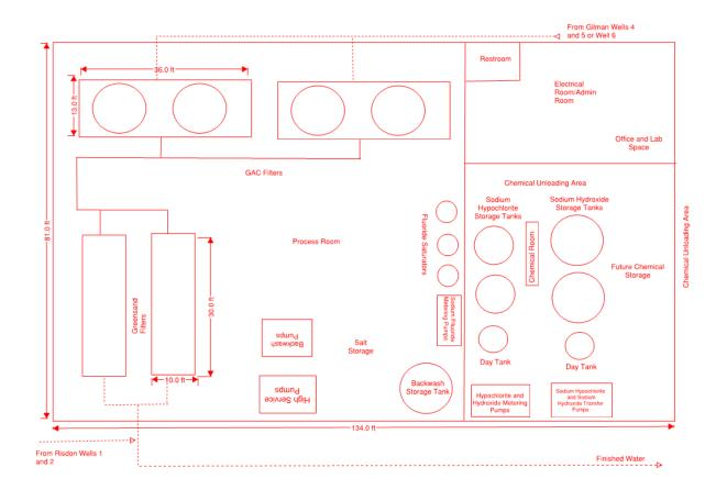
Figure 3. Conceptual Centralized Treatment Facility Layout
