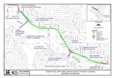
This project will be designed and constructed to control combined sewer overflows (CSOs) to the Lake Washington Ship Canal, as approved by both King County's and City of Seattle's respective Consent Decrees. SPU is responsible for completion of the construction, subsequent operation and maintenance, periodic repair, replacement and permitting of the Ship Canal Project.
