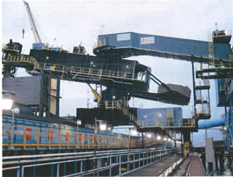
Figure 13: New Travelling Shiploader for Mineral Concentrates
