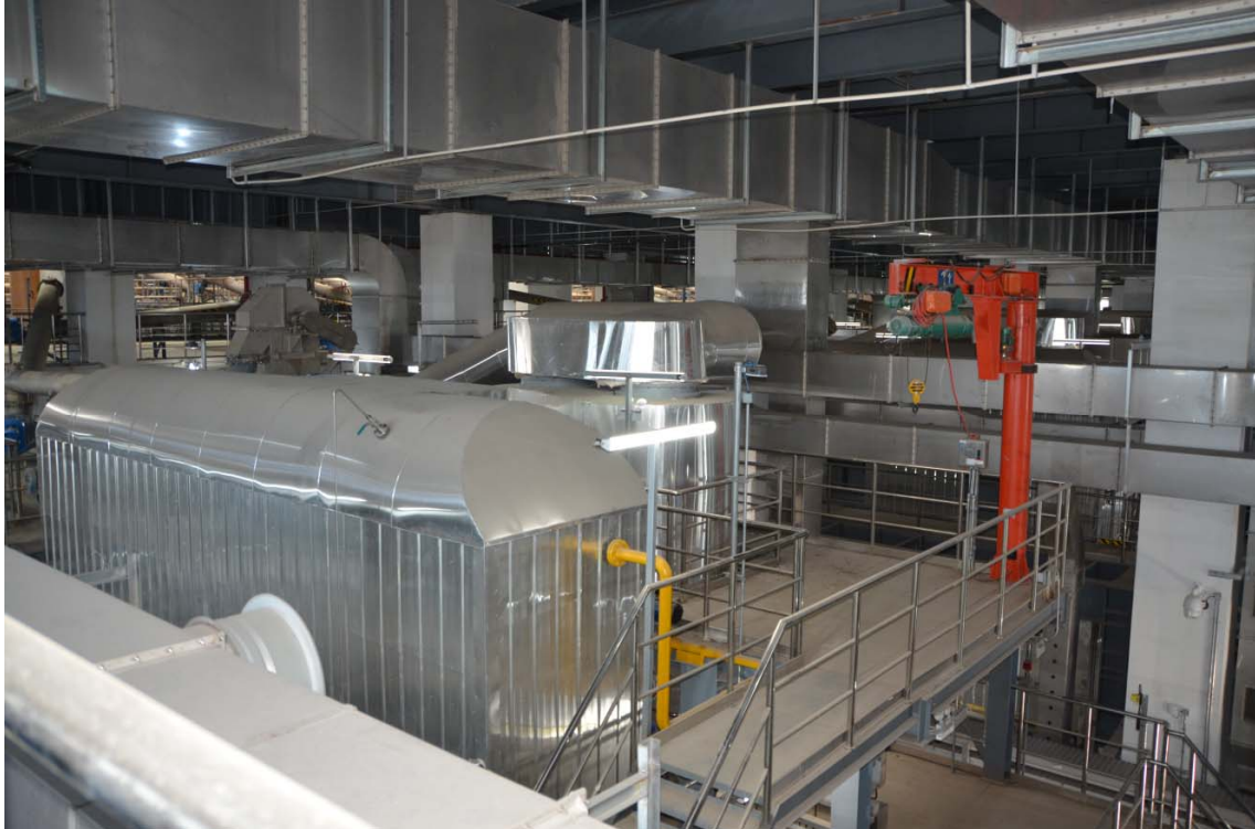
Steam Heated Fluid Bed Drying System, FDS 9.0 Bailonggang China
