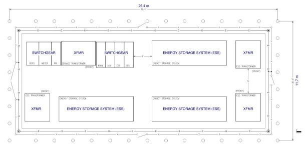
Figure A4: Electrical Equipment at Kenmore or Shilshole for Round-Trip Full-Electric Service
