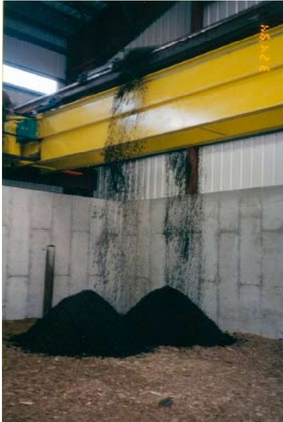
Processing floor, Screened humus is delivered by over head conveyor equipped with traveling discharge
