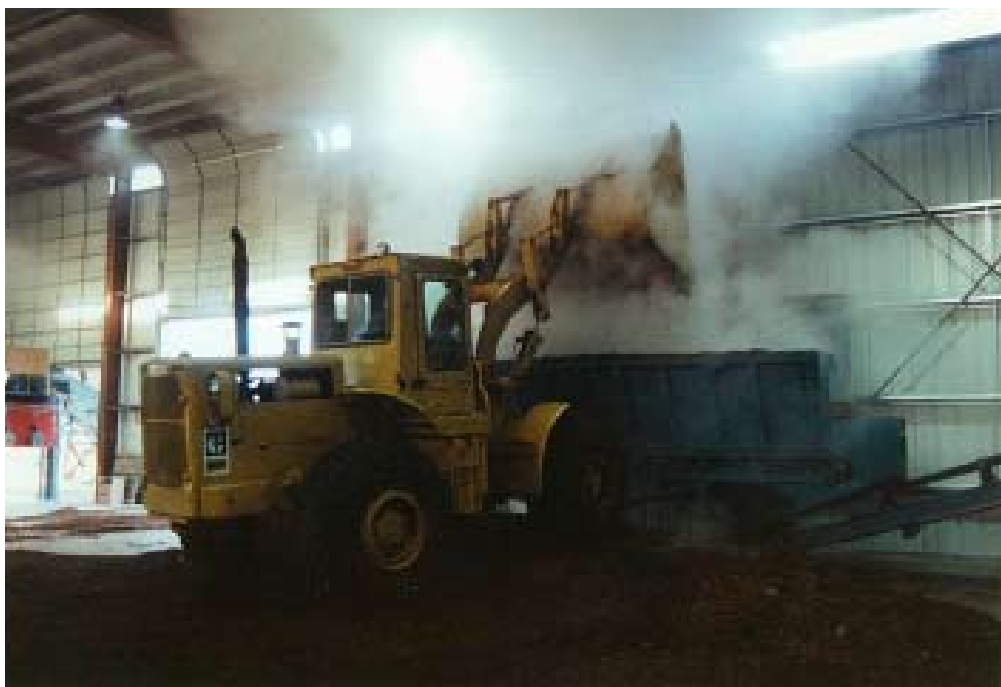
Processed humus is deposited into the hopper of the rotary drum screen for screening
