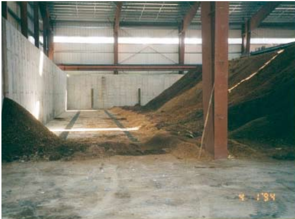
This is an empty Loop ready to be filled with 1,000 cubic yards (There are 10 loops in this building, for a total of 10,000 wet tons of processing)
