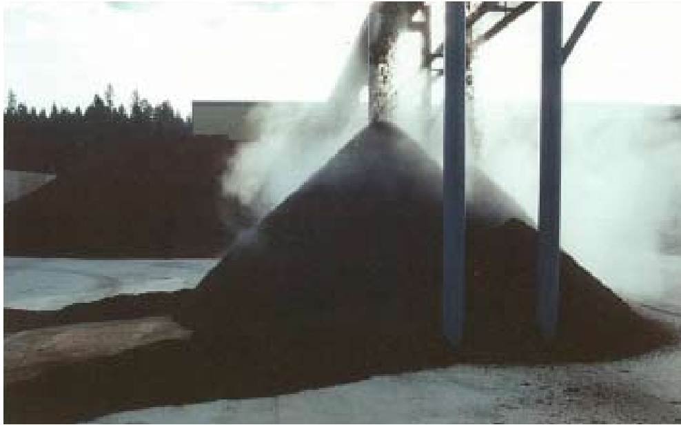
After specific number of weeks, the screened humus is deposited into the curing area.
