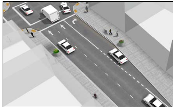
Example of a right turn pocket.
