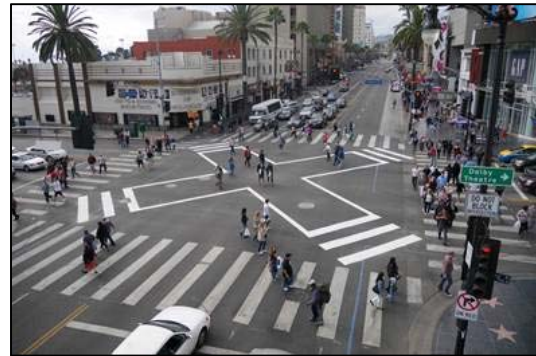
An example of a pedestrian scramble.
