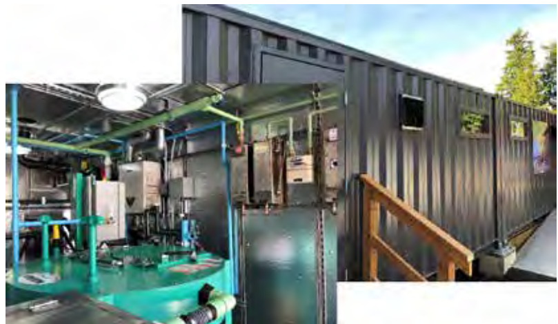
Example of a small anaerobic digester in Redmond (Photo courtesy of Impact BioEnergy, Inc.)
