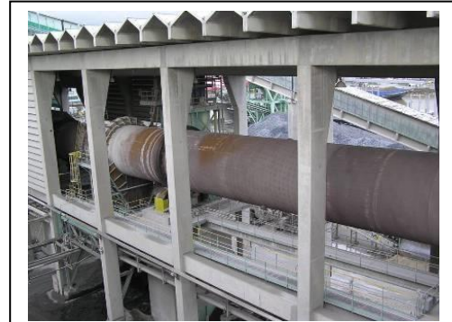
A portion of the 540 ft. long wet process kiln at Lafarge Seattle, formerly the Ideal/Holnam Cement plant. (pavementinteractive.org)
