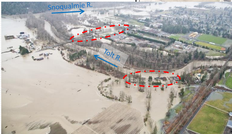
Levee breach and SR 203 flooding, Jan. 2009
