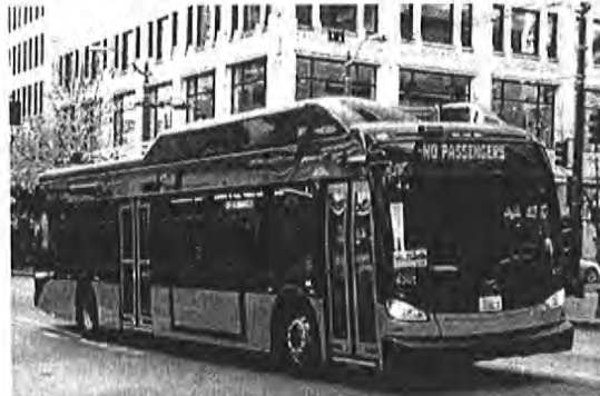
New 40-foot trolley with enhanced energy efficiency, regenerative braking and the ability to travel limited distances on a battery.
