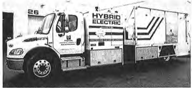
This hybrid service truck supports field preventive maintenance on fleet vehicles and equipment. The truck uses the hybrid battery to operate the air compressor and 12 volt/110 volt electrical systems making it unnecessary to run the engine when carrying out service operations.
