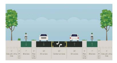
[Note: bike lanes are slightly widened to account for more traffic and differential speeds on the hill. Also, in places where a median island exists instead of the center turn lane, the median island would be kept.
