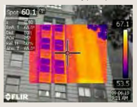
Figure 8 Infrared photo shows heat loss (yellow) through panel section on right compared to high efficiency windows on the left. Outdoor Temp is 53 degrees in this picture.
