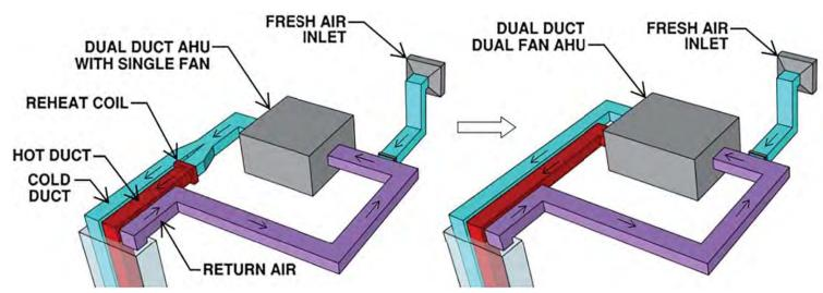
The existing ductwork will be utilized to deliver hot and cold air to the dual duct terminal units on each floor. This ductwork and sheet metal will need to be cleaned, re-sealed, re-insulated, and pressure-tested prior to connection to the new air handling units.
