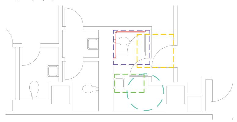
Diagram showing the required ADA clearances for toilets and lavatories superimposed over a drawing of the existing toilet room configuration at the jury deliberation rooms.
