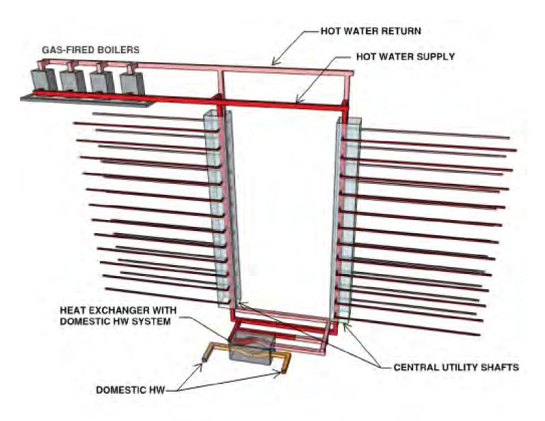
Heating Hot Water System Diagram
