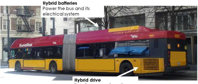
Transfers power from the batteries to the rear wheels
