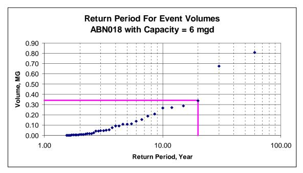
Figure 5-7. Volume vs. Return Period Curve
