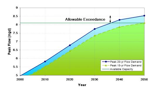
Figure 5-5. Allowable Exceedance at 2050 Saturation Flow Demand
