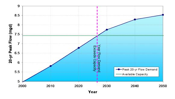
Figure 5-4. Determination of Exceedance and Year Exceeded
