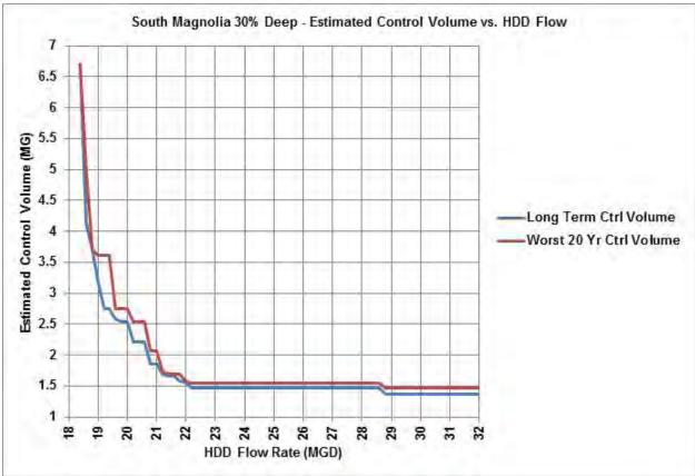
Figure 4-3. CSO Storage vs. Downstream Conveyance (HDD) Capacity
