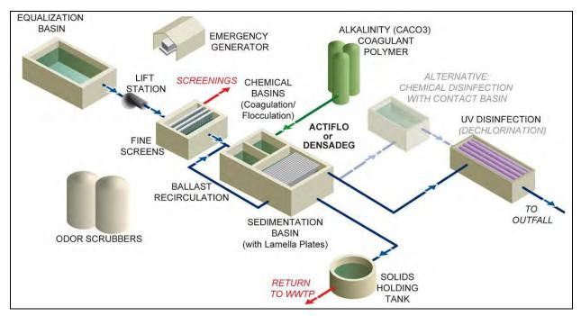
Figure 4-5. Sample Process Flow Schematic for Ballasted Sedimentation
