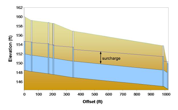
Figure 5-3. MOUSE Pipe Profile With Surcharging
