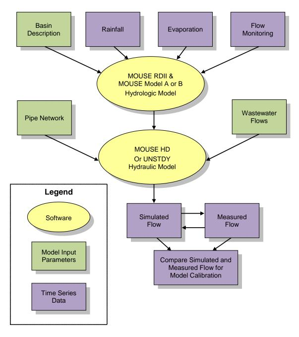
Figure 3-1. MOUSE Hydrologic and Hydraulic Model Components
