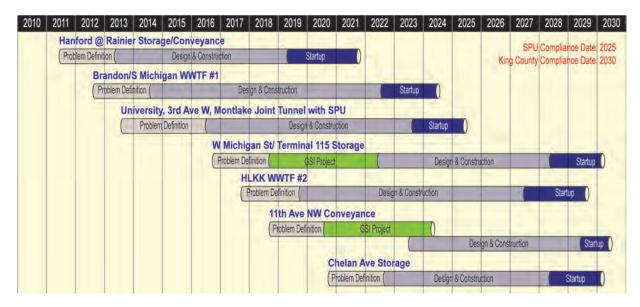
Figure 7-5. Joint-Tunnel Project Sequence Alternative
