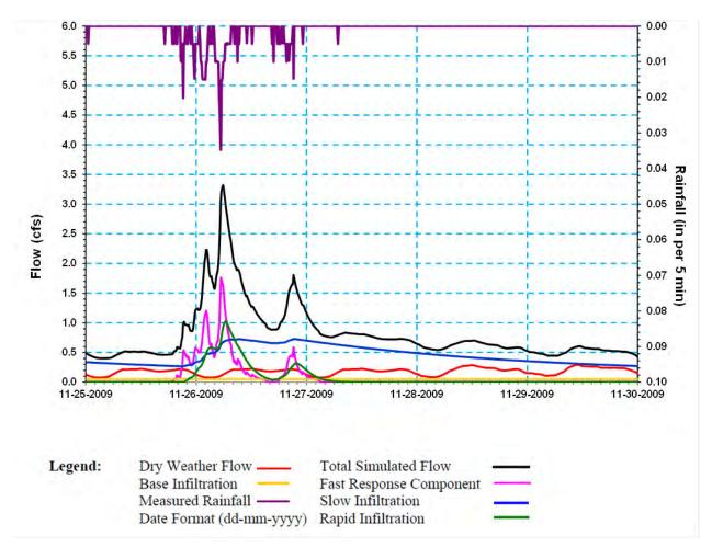
Figure 3-9. Simulated Flow Components in a Combined System
