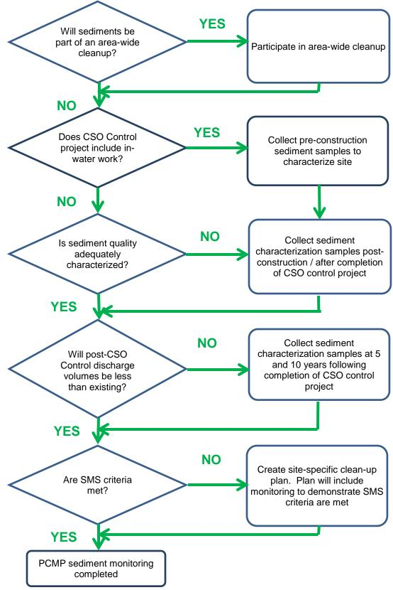
Figure 3. PCMP Sediment monitoring flowchart
