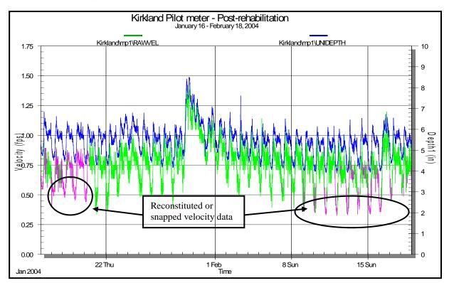
Figure B.3 - Hydrograph of reconstituted velocity data
