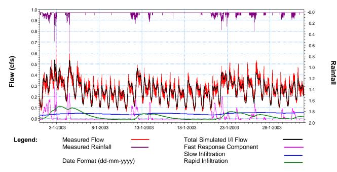
Figure 3-8. Comparison of Modeled Flow Data to Measured Flow Data
