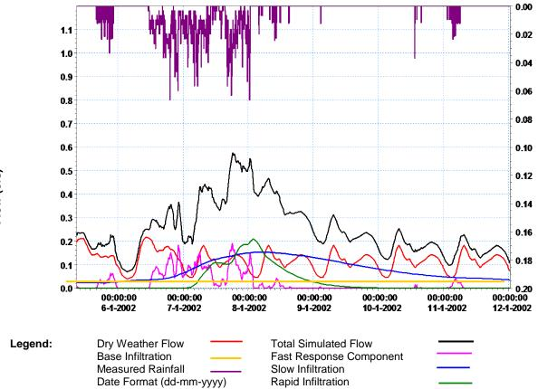
Figure 3-10. Simulated Flow Components in a Separated System
