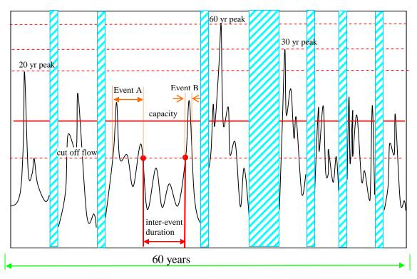
Figure 5-6. Schematic of a 60 year hydrograph
